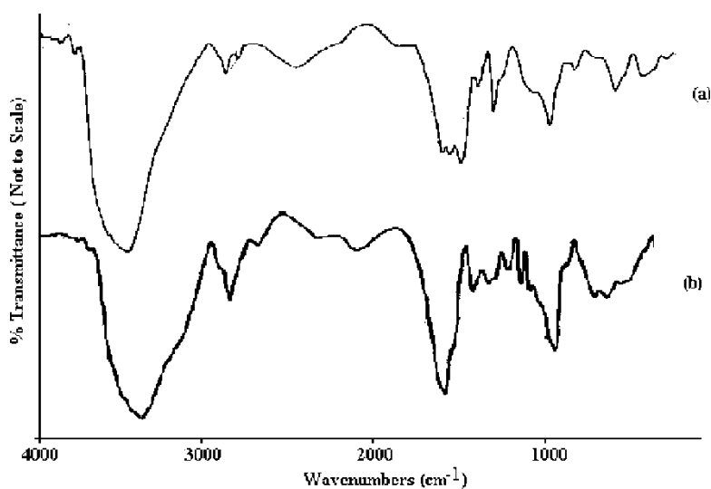
Figure 3. IR spectra of (a) Plain hydrogel sample; (b) Model drug vitamin B 12 loaded hydrogel sample.
